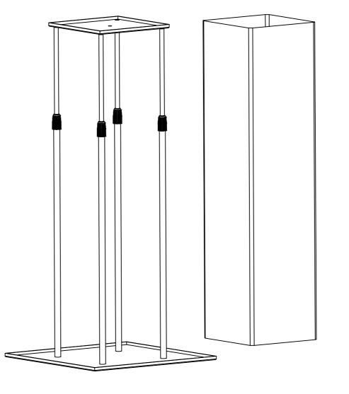
The height of each pole is adjusted by rotating the locking handle; anti-clockwise to loosen the clamp, clockwise to tighten.
