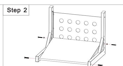
Mount the mixer shelf between the two L-shape legs after you have selected the desired mixer angle from the 5 mounting positions and insert the bolts and washers as shown above.
