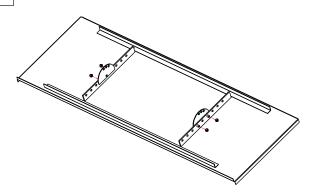
Now position and bolt in the two steel circular plates to the top plate; it is at this point that you select the depth of the top shelf before you bolt on these plates. IMPORTANT: these circular plates must be mounted on the INSIDE of the rail and the holes in the circular plates MUST FACE towards the FRONT edge of the top plate – as shown in the image above)
