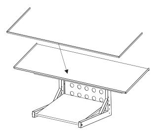
Attach the rubber protection edging to the lip of the top plate. You may need to lay the edging in place first and bend the corners to assist the fixing around the corners.
