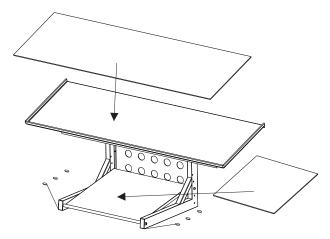
If required, attach the double sided foam EVA pads to the top and bottom panels and attach the non-slip rubber feet to the underside of the frame as shown.
