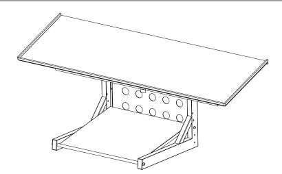
Now securely tighten all the bolts - BUT DO NOT OVERTIGHTEN AND THREAD THE SOCKETS.
